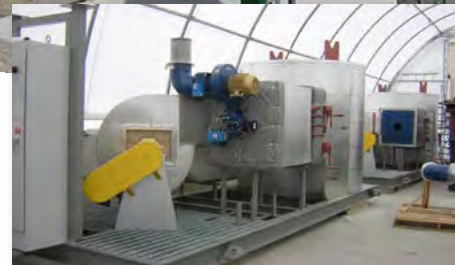
Model RBO Recirculation Fan for Melting Plastic
